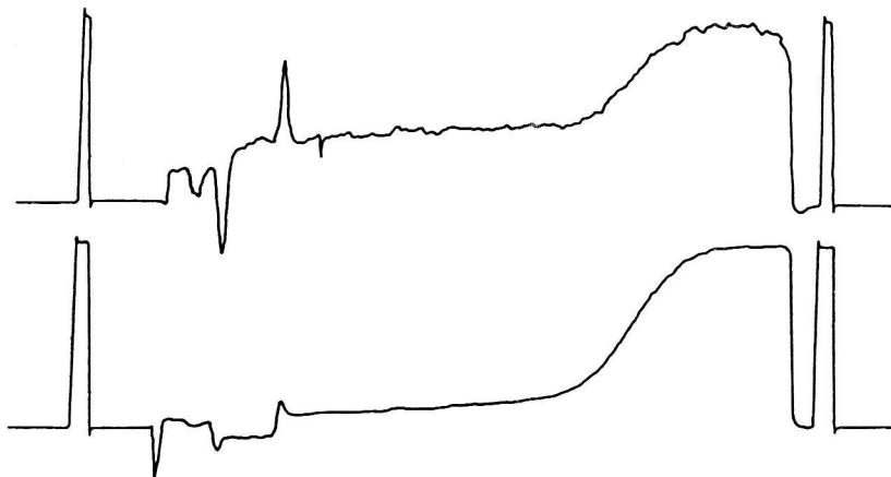
Fig. 4. Cosedimentation diagram for methyl-malonyl mutase and its cofactor (offset toward the top) scanned within 2 min of each other. The center of the sedimenting boundary is virtually the same for both, confirming that under the solvent conditions used (50 mM-Tris/HCl, pH 7.5 + 5 mM EDTA) the cofactor is bound to the protein. These scans were obtained from an MSE Centriscan, monochromator wavelength = 295 nm (bottom), 608 nm (top); rotor speed = 44,000 rpm; temperature = 20.0°C, c^\circ = 0.7 mg/mL.
