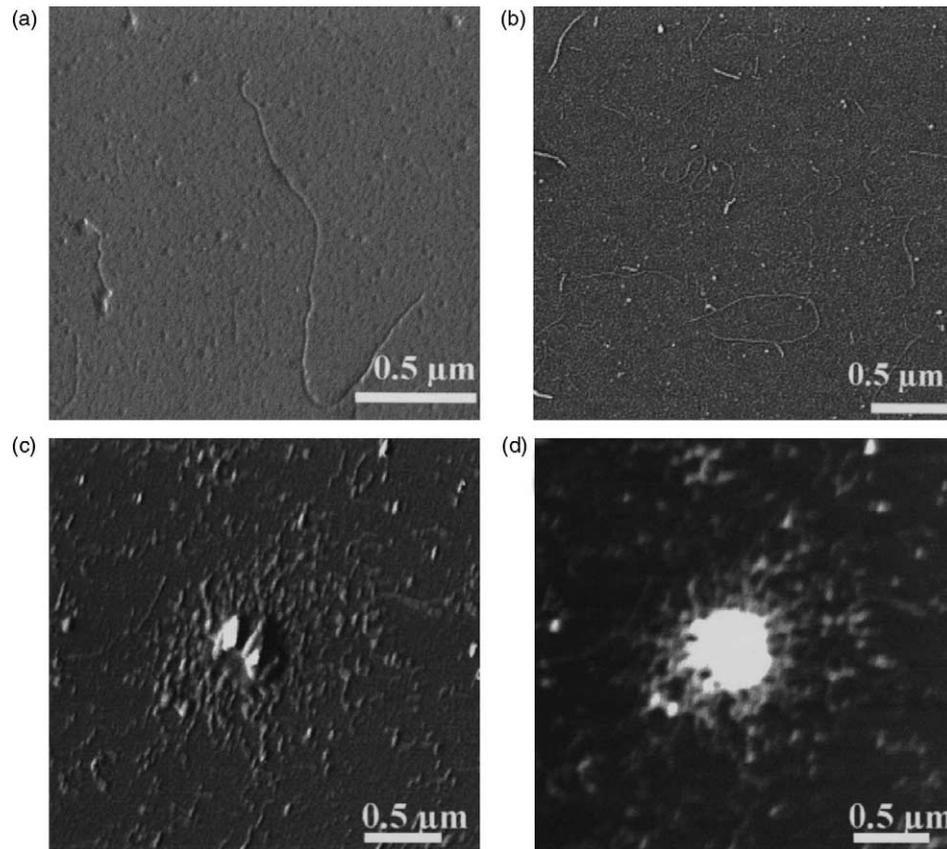
**Fig. 6.** Atomic force microscopy image of mucin, chitosan and chitosan–mucin complex. (a) Mucin by itself; (b) chitosan; (c) and (d) chitosan–mucin complex. All images taken in ‘phase’ mode apart from (d) which was taken in ‘tapping’ mode. From Deacon *et al.* (2000).
