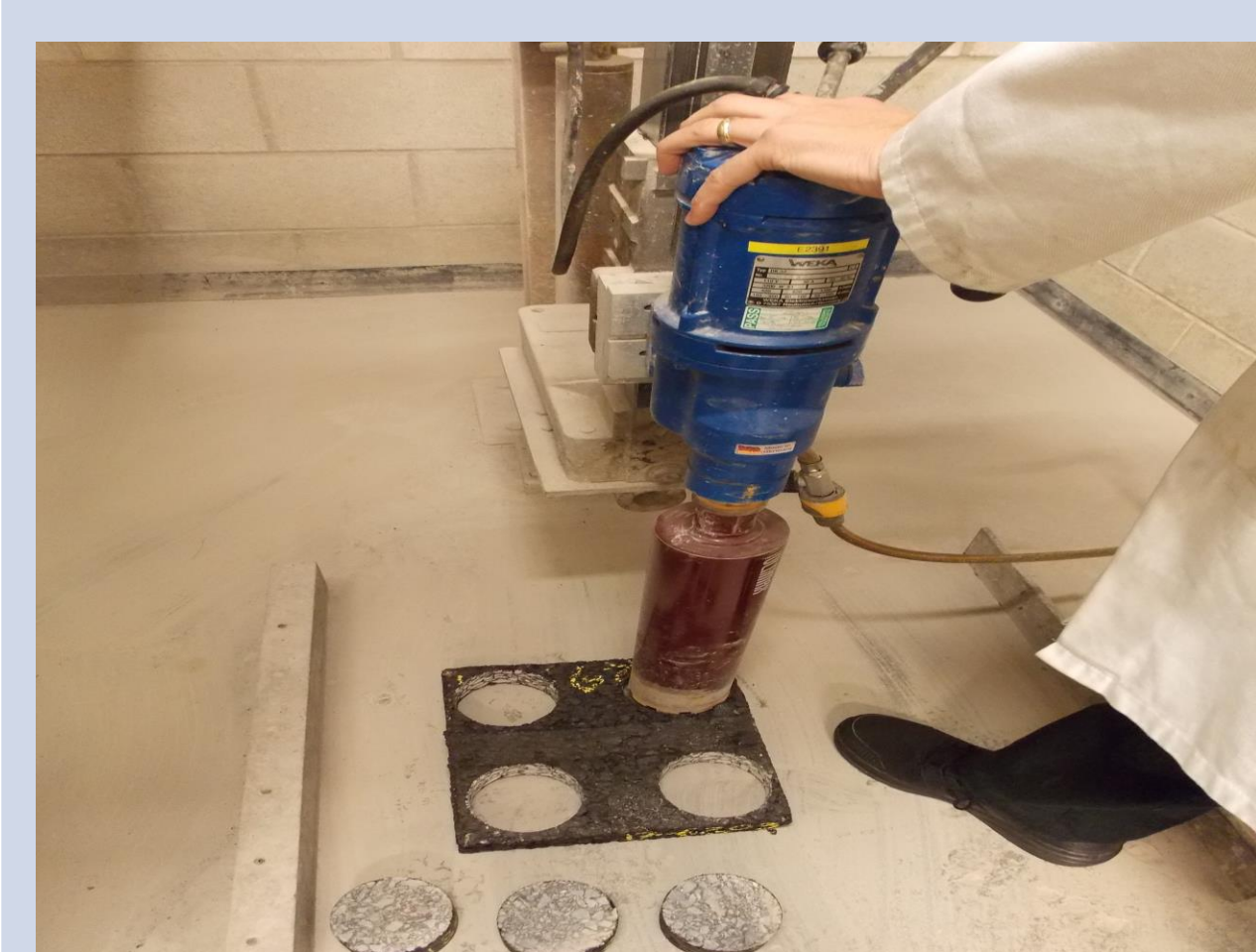
Coring of Asphalt Specimens
