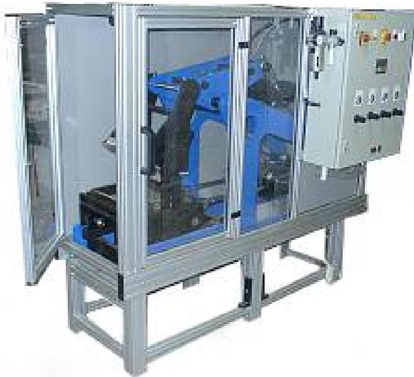
Figure 5.2 – Roller slab compactor.
