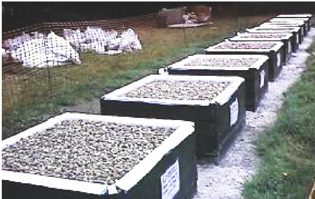
Figure 7-2: Constructed lysimeter field
