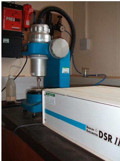
Figure 4-5: The Dynamic Shear Rheometer used during the mastic testing
