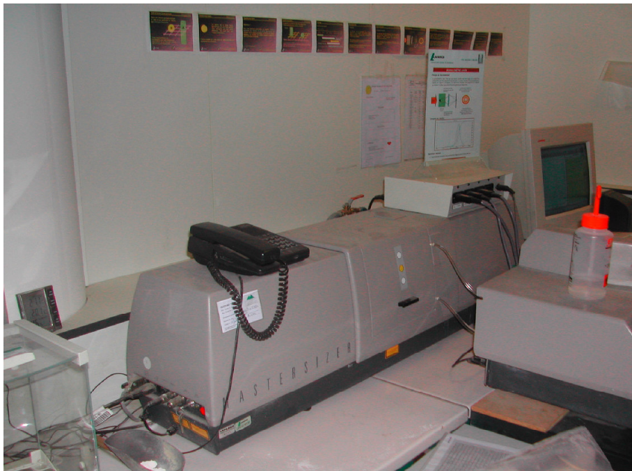
Figure 3-3: Equipment used for measuring particle size distribution of the fillers - laser diffraction technique
