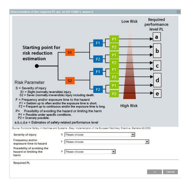
In assessing the likelihood of a person entering a designated laser area, the Severity is classed as S2 (Severe), the Frequency as F1 (seldom up to often and/or exposure time is short) and the Possibility as P1 or P2, depending on the set up within the laser room. This gives a required performance level of C or D.
