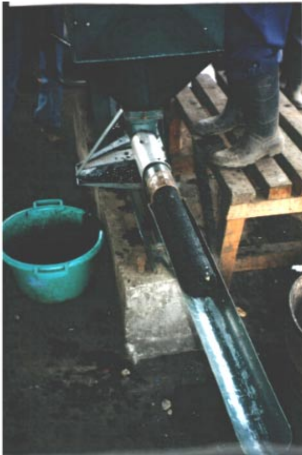
Figure 2.1. LP piston press developed by ITDG EA.
