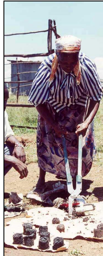
Figure 2.4. Briquetting 'tongs' being used in Kenya.
