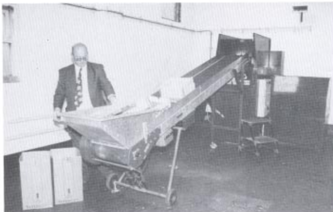
A conveyor helps ease the loading of dry waste material into the Brickman 300 briquetting press at Leigh Infirmary, maintaining throughput at an optimum level.
