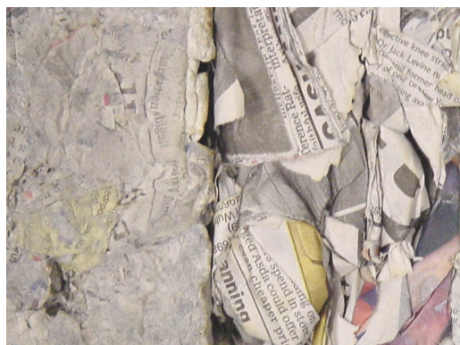
Fig. 3.23: Briquette structure when soaked for 0 and 473 hours. (0 hours on right)
