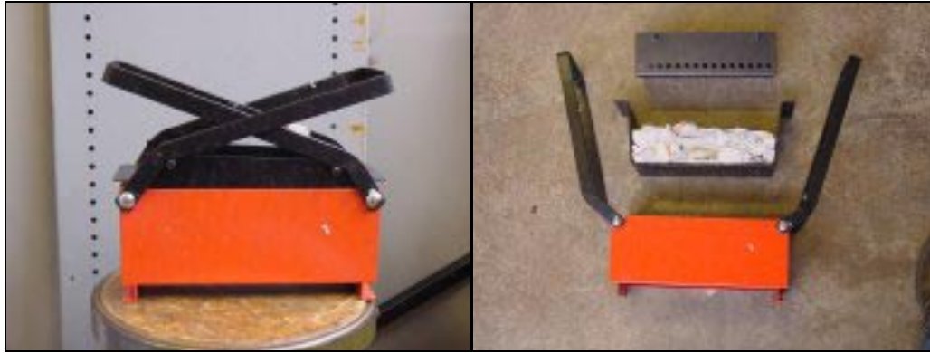
Fig. 3.1. Hand operated lever press from CAT. Figure on right shows compacted briquette in position
