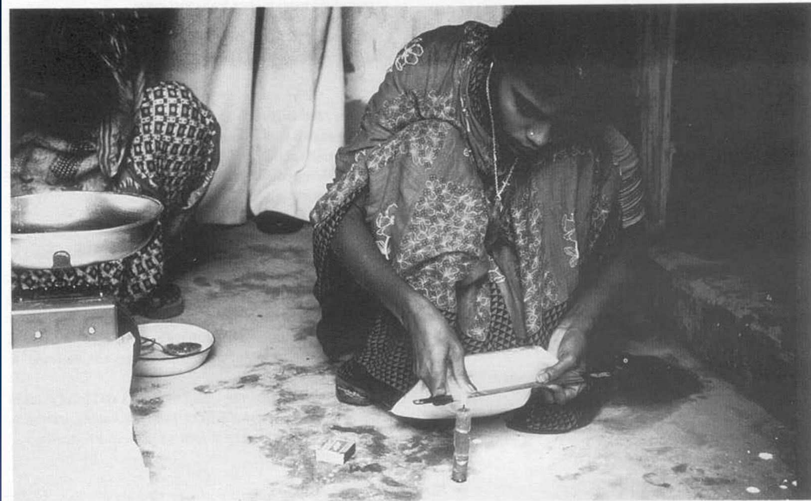
Sealing plastic bags with a candle and hacksaw blade
