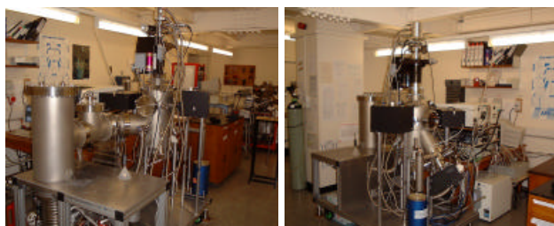
Figure 1. The “Nottingham Star Dust Machine” for studies of molecular ice surfaces in ultrahigh vacuum at cryogenic temperatures.
