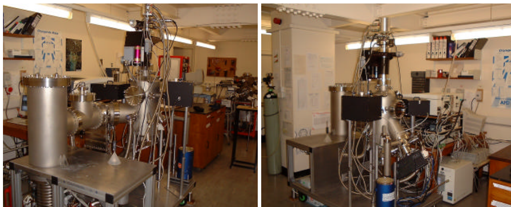
Figure 1. The Nottingham Apparatus for studies of molecular ice surfaces in ultrahigh vacuum at cryogenic temperatures.
