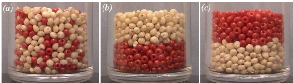
FIG. 2. The separation of millet and insulating beads. (a) After vibration at 10 Hz for 300 s in zero magnetic field. Middle; (b) after vibration for 30 s with BdB/dz=-730 \text{ T}^2 \text{ m}^{-1} ; (c) after vibration for 30 s with BdB/dz=+1000 \text{ T}^2 \text{ m}^{-1} .
