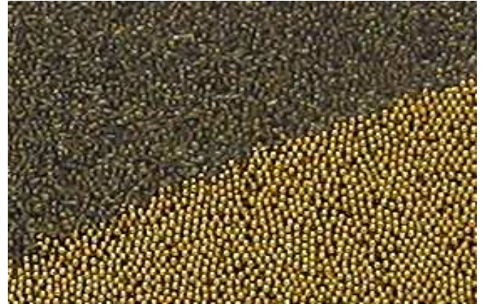
Figure 2. A close-up view of the separated boundary between bronze and bismuth particles ( 75 - 90 \mu\text{m} ) following vibration in air at \Gamma = 1.5 , f = 10\text{Hz} , -B dB/dz = 500 \text{ T}^2\text{m}^{-1} for 120s
