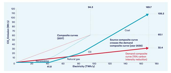
Figure 3. Carbon-energy diagram for year 2030, with 117.5 TWh from zero-carbon power plants, leaving just 8.5 TWh from coal-fired power plants
