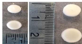
Fig. 2: PCL-M (top) and PGS-M (bottom) scaffolds after natural shrinkage in methanol solution.
