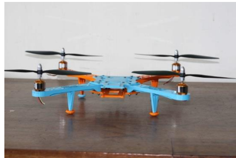
Locally assembled UAVs and other accessories made from 3D-printed parts
