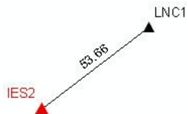
Figure 4: A long baseline used during static test TS8. The rover site location (IES2) with a reference station (LNC1) located 53.66km away.
