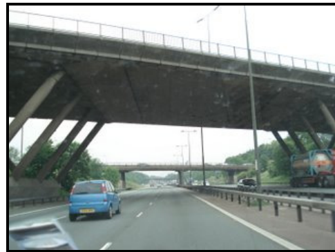
Figure 11: View of one flyover bridge from the test car during TK1 (M1 Motorway). Such bridges caused GPS signal blockages along the M1.
