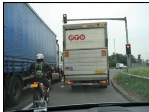
Figure 12: Lorries on the M1 Motorway blocked GPS signals and potentially caused dynamic multipath.
