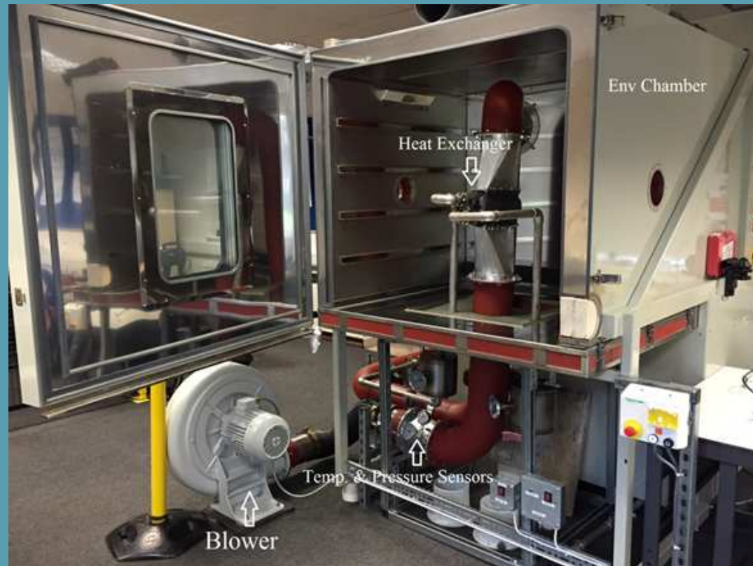
The heat exchanger life testing rig at the centre laboratory
