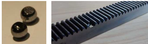
Damaged balls and gear rack:
