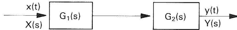
Figure 8. Two non-interacting systems, G_1(s) and G_2(s) , in series, with inputs x(t) and X(s) and outputs y(t) and Y(s) .
