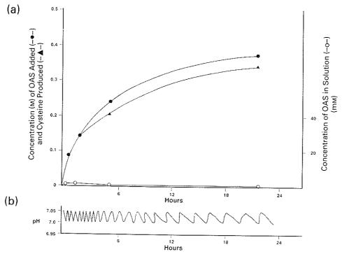
Figure 16. 1.-Cystcine production by O-acetylserine sulphydrylase (OASS) with 2·3 M sodium hydrosulphide as substrate. (a) (●) Cumulative amount of O-acetylserine (OAS) added. (▲) Cysteine and cystine produced. (o) OAS actually present in reaction mixture. (b) pH profile of bioconversion (Hsaio and Wei, 1987).
