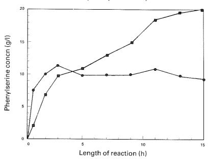
Figure 5. Fed-batch production of β-phenylserine from glycine and benzaldehyde with SHMT. Conditions: 35°C, pH 7, 100 g/l glycine, 5000 units/l SHMT (Walter and Bull, 1987). threo (———); erythro (————).
