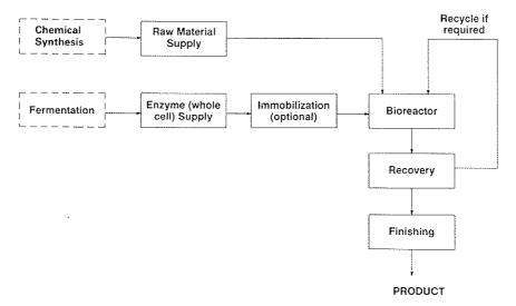
Figure 1. Elements of a typical manufacturing process for the enzymatic production of amino acids.
