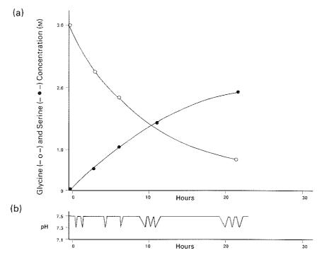
Figure 4. SHMT bioreactor results for enzymatic synthesis of serine  $(- \bullet -)$  from glycine  $(- \circ -)$  and formaldehyde. The change in amino acid composition with time is shown in (a), and the pH profile is shown in (b). From Hsiao and Wei, 1986.
