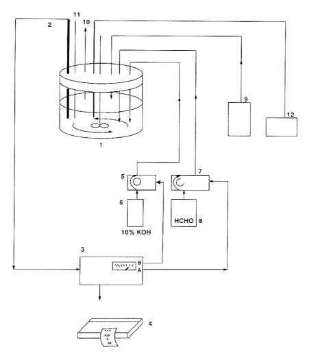
Figure 3. Bioreactor configuration used for enzymatic synthesis of serine with SHMT: 1. Bioreactor; 2. pH electrode; 3. pH controller; 4. Recorder; 5. P-1 pump; 6. 10% KOH; 7. P-1 pump; 8. Formaldehyde solution (37%); 9. N<sub>2</sub> tank; 10. N<sub>2</sub> outlet; 11. Sampling tube; 12. Temperature control. From Hsiao and Wei, 1986.
