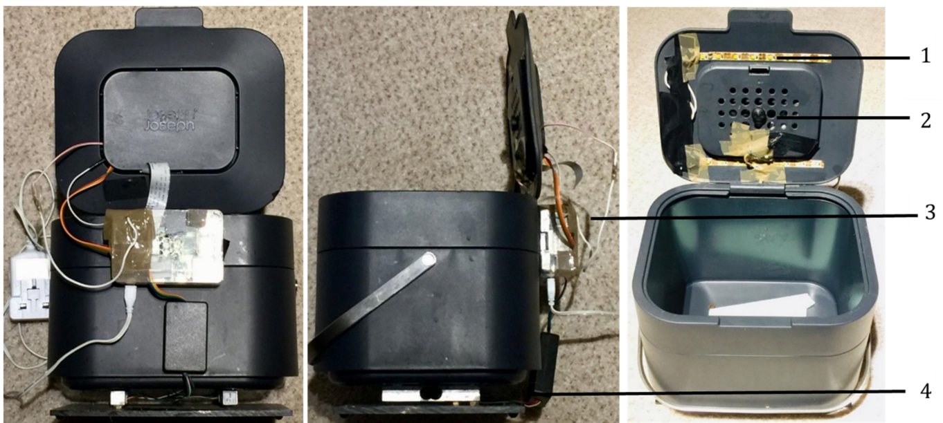
Figure 2. The smart bin. The smart bin is comprised of a 4-liter caddy with dimensions 23.5 \times 19.7 \times 16.1 cm. In the lid is a light bar (1) and a motion sensitive camera (2), that when the lid is lifted is programmed to take 6 photos. These are wired to a mains-powered, Raspberry Pi single board computer (3). This is connected to the household Wi-Fi and data is recorded remotely. Finally, the Raspberry Pi signals a set of weighing scales (4) to record the weight of the bin each time the lid is opened.
