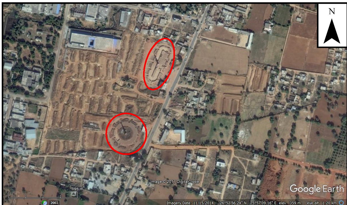
Fig. 2. An image featuring two brick kilns. One is a traditional Bull's Trench Kiln (BTK) and the other is a circular kiln. Surrounding these kilns is a number of clay fields that are used in the production of the bricks themselves before the firing of the bricks in the kilns. These fields are commonly found close to the kilns although sometimes they are not directly adjacent to the kilns.
