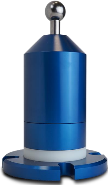
Calibrated spherical artefact [1]
