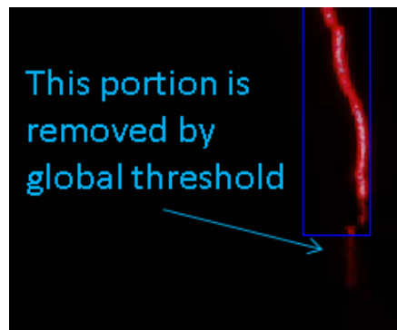
Figure 109: Omitted portion when applying global thresholding
