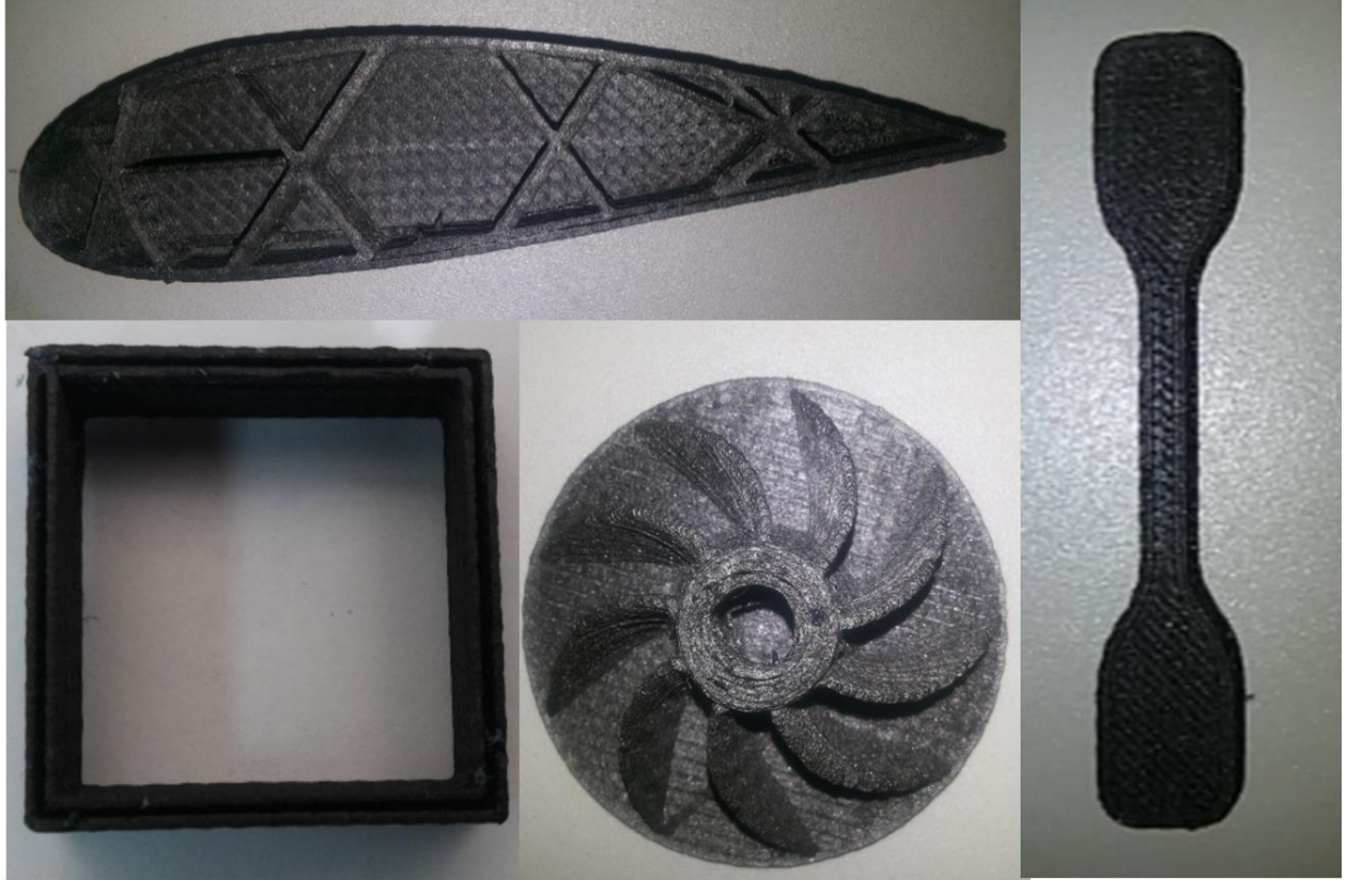
Figure 20: Sample parts fabricated with chopped fiber composite
