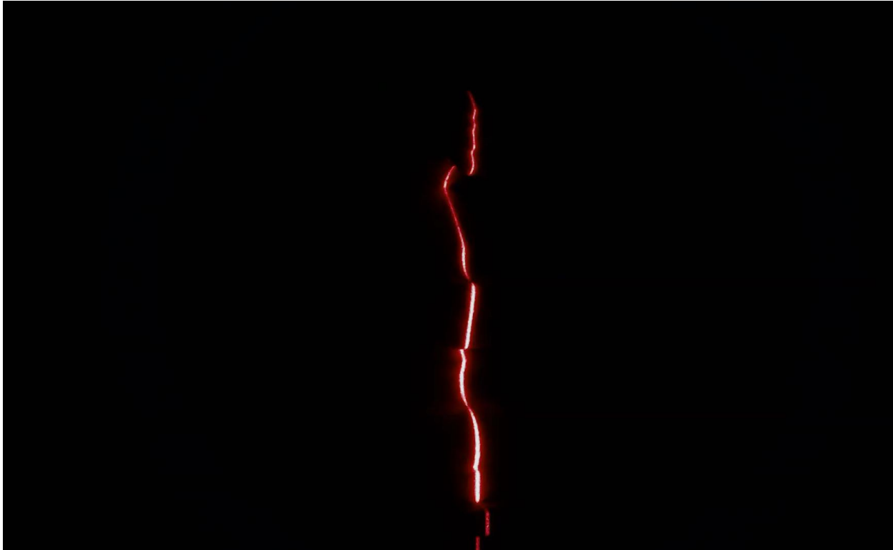
Figure 85: Raw image obtained from the image sensor during the scanning of a knight piece
