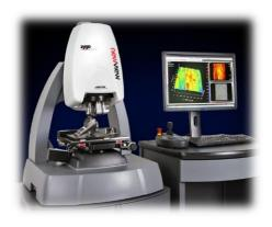
The Zygo New View<sup>™</sup> 8300 coherence scanning interferometer is a 3D optical surface profiler and provides powerful versatility in non-contact optical surface profilina. All measurements are nondestructive, fast, and reauire no sample preparation. Advanced software tools
