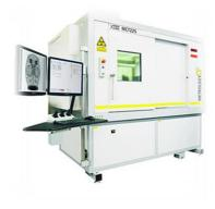
The **Nikon MCT 225** is an X-ray computed tomography system for metrology of the external and internal features of samples. The instrument takes a number of 2D X-ray images at varying angles around the sample to capture the internal and external geometries of the sample. These 2D images are then reconstructed to form a 3D model, which can then be used to perform dimensional
