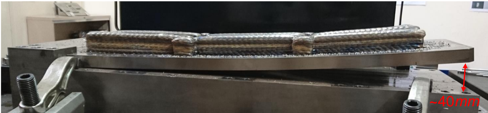
WAAM produced part tilts up due to the residual stress
