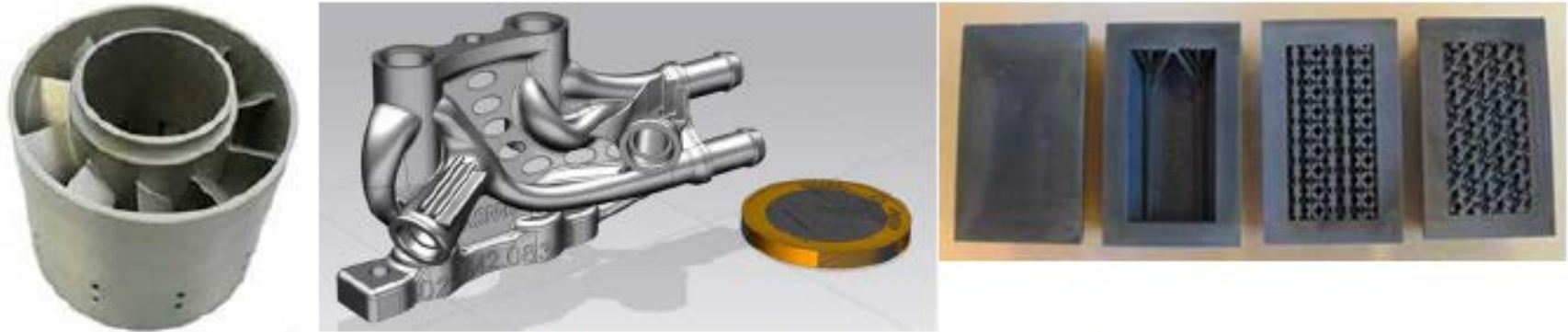
Figure 2.1a: Proposed applications to guide the PAM 2 research: an impeller (left, GE), a typical manifold for conditioning water, with interfaces for temperature sensors in TiAl6V4 (middle, ASML) and prototypes of injection moulding tool inserts in maraging steel (right, LEGO, alternative designs with lattice structures to save materials & speed up the process)
