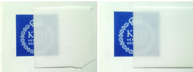
Fig. 35. Pictures of the sintered alumina (left) and zirconia (right) single layer samples, with a thickness of 186 \mu\text{m} and 212 \mu\text{m} , respectively. Note the fuzziness of the KTH logo when the light is transmitted through the samples.
