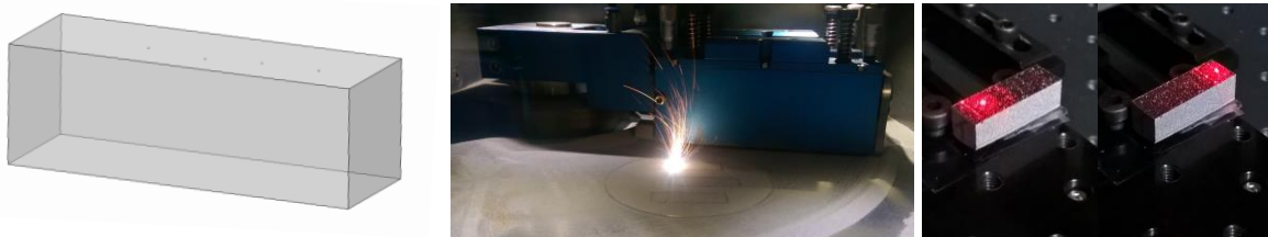
Figure 4 - Schematic of block with seeded defects (left), SLM50 processing of samples (centre) and photographs showing start and end laser positions for LU (right).
