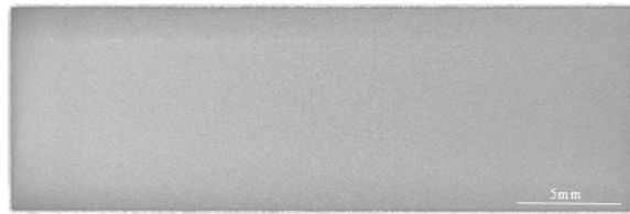
Figure 8 - XCT image of AM solid block sample (x-y plane at 250 \mu\text{m} from top surface).
