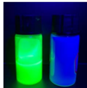
Solutions of caesium lead halide perovskite nanocrystals with different halide contents
