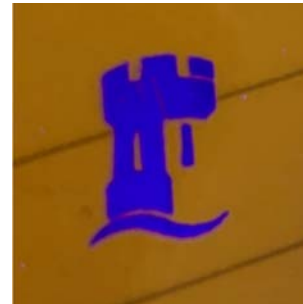
University of Nottingham logo printed using caesium lead halide perovskite nanocrystal ink
