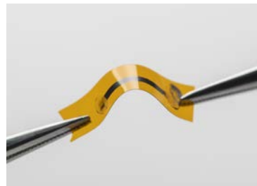
Fig2: Graphene layers printed on a flexible substrate.
