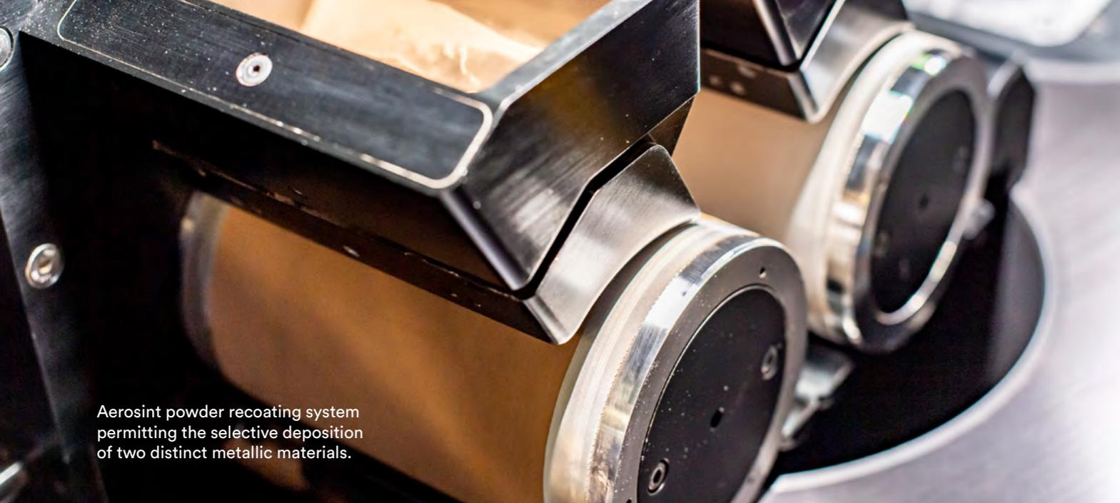
Aerosint powder recoating system permitting the selective deposition of two distinct metallic materials.
