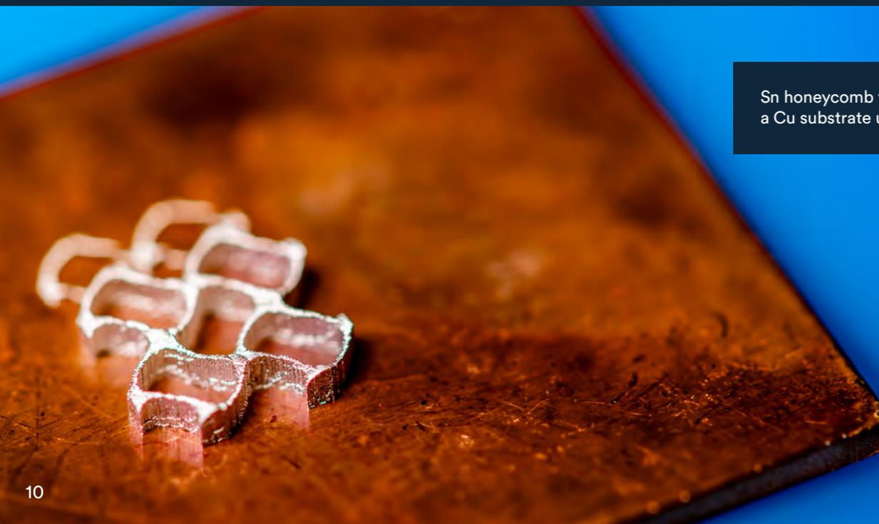
Sn honeycomb test specimen created on a Cu substrate using the MetalJet process.
