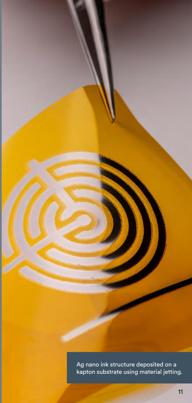
Ag nano ink structure deposited on a kapton substrate using material jetting.
