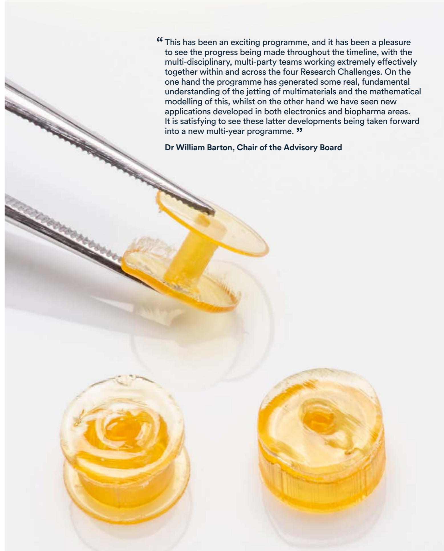
Image: 3D-printed pills will allow digital design of medication release. In this image, the insoluble core and barriers used to control the drug release of a 3D-printed pill.
