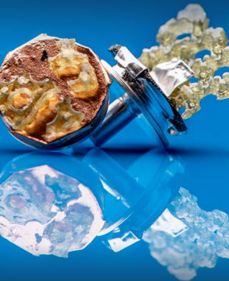
Image: Multiple versions of 3D-printed finger stent exemplar on the SEM stubs.
