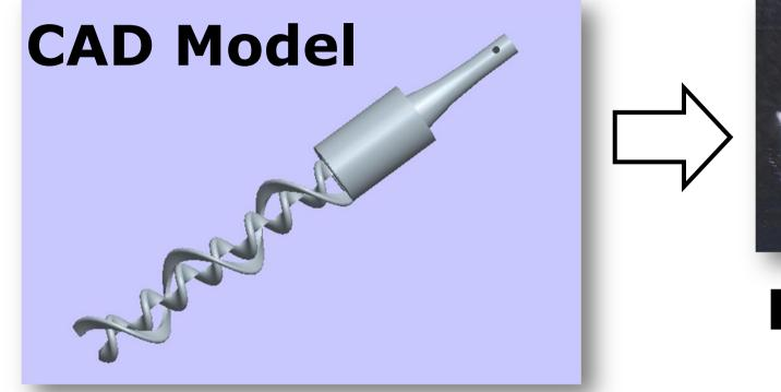
impeller The was fabricated using a 4-axis machine tool IN aluminium initially as a test cut and finally in 316L stainless steel for the final impeller.
