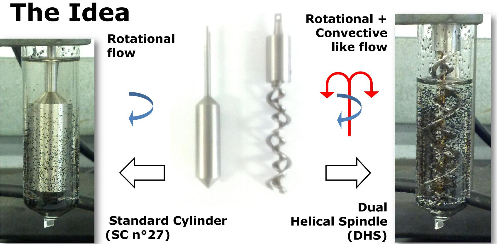
Common systems for measuring viscosity of bitumen, Concentric cylinders with Standard cylinders (SC) as impellers, are not able to prevent phase separation. This does not allow for an even distribution of tyre rubber particles within the bitumen matrix, so neither mixing process nor viscosity measurements will be accurate.
