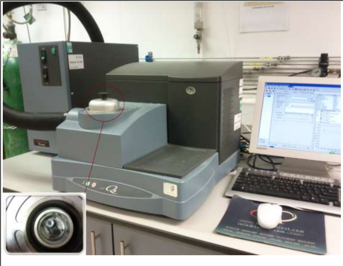
Figure 3-4 A TA Instruments Q10 Differential Scanning Calorimeter
