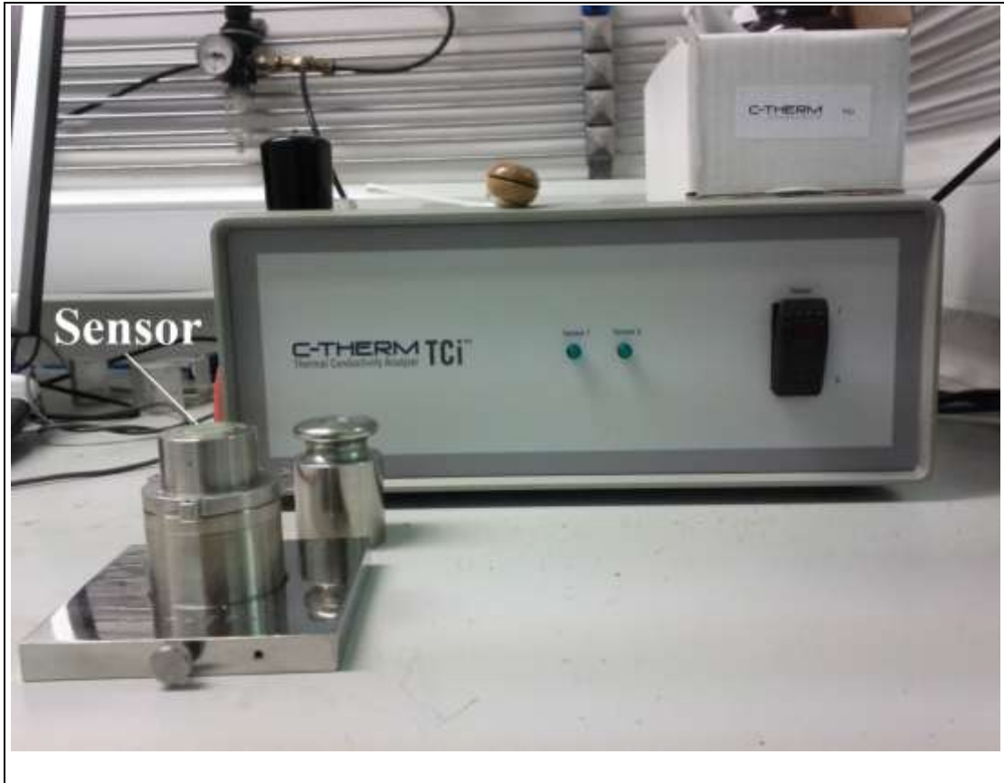
Figure 3-3 Mathis TCI thermal conductivity analyser
