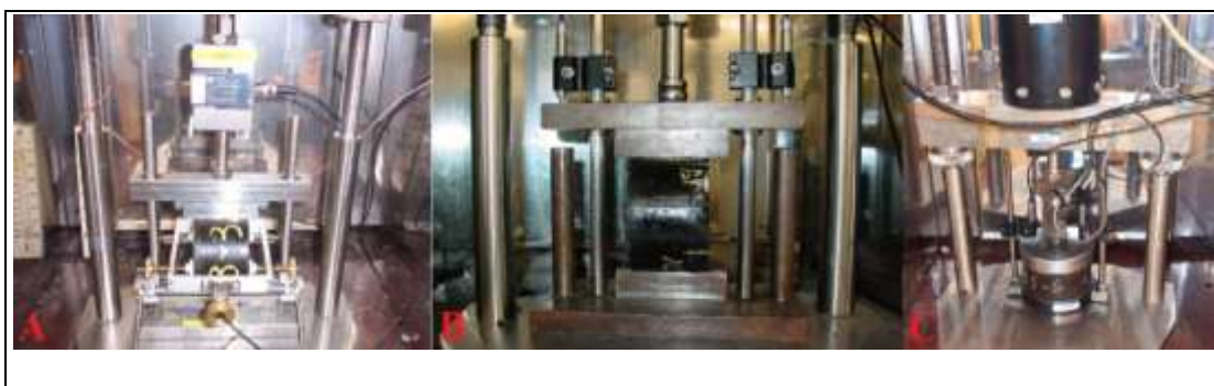
Figure A-2 Different Modes of Testing in the NAT, (A) ITSM, (B) ITFT, (C) RLAT
