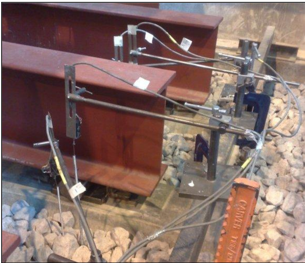
Figure 5.7 Potentiometers arrangement in RTF Test 9
