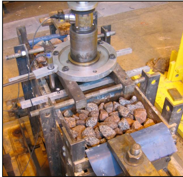
Figure 6.1 (b) The box test set-up
