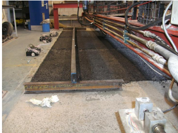
Figure 7.16: PTF surface layer
