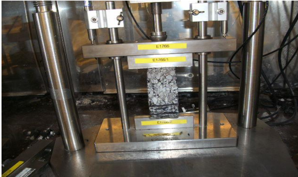
Figure 3.7: Test configuration for ITFT in NAT
