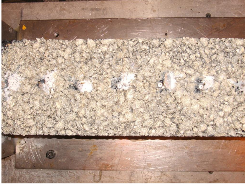
Figure 8.18: Specimen with proprietary SAMI A after test (left)
