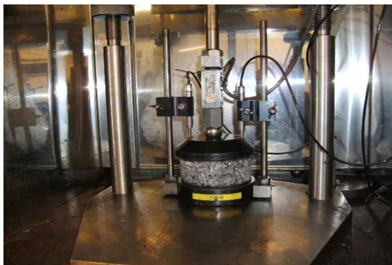
Figure 3.9: Test configuration for RLAT in NAT
