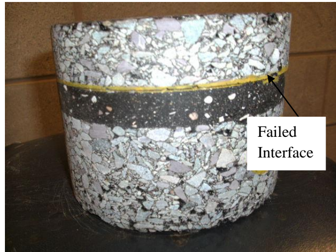
Figure 4.11: A typical failed interface after test
