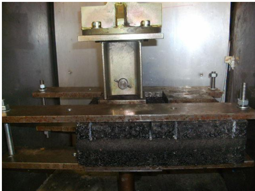
Figure 4.12: Pull-off test set up
