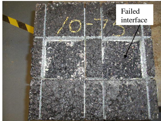
Figure 4.15: A typical failed interface after test
