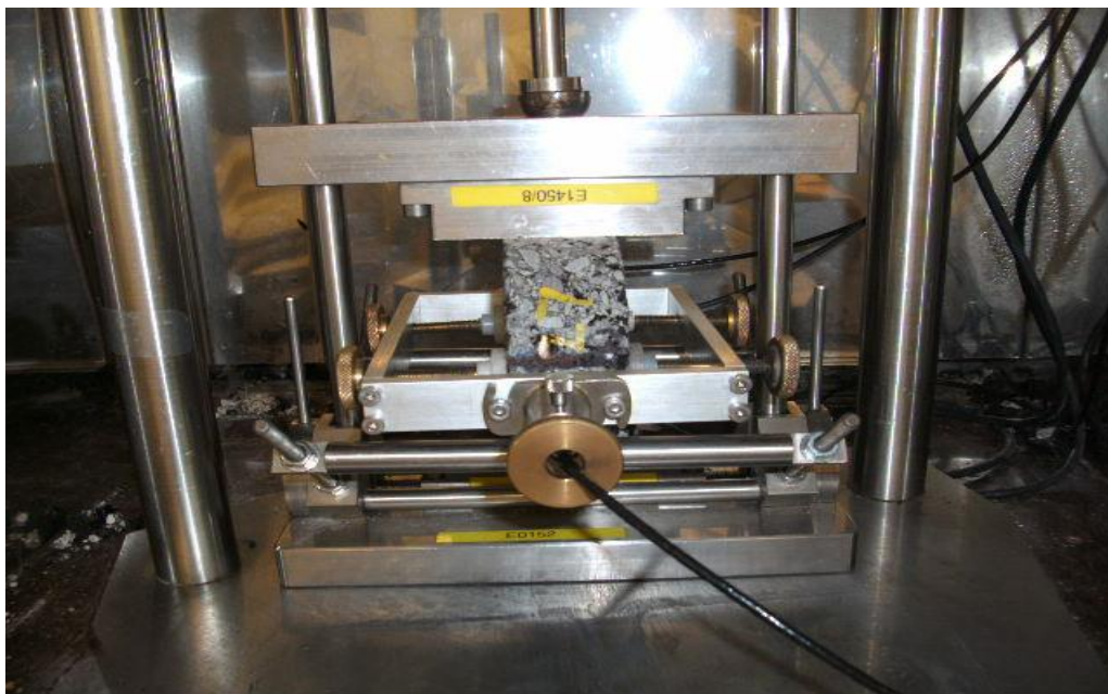
Figure 3.6: Test configuration for ITSM in NAT
