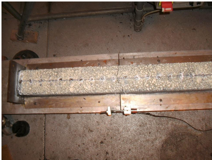
Figure 8.47: Specimen with sand asphalt at the end of test
