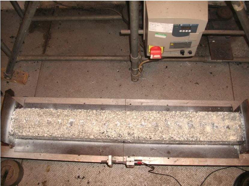
Figure 8.39: Specimen with proprietary SAMI D at the start of test
