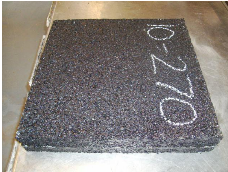
Figure 5.2: A typical 500 mm by 500 mm slab
