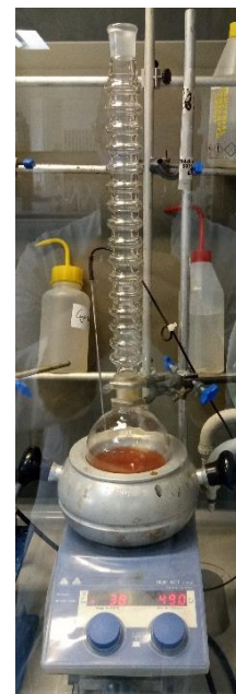
Figure 4. Waterless condenser setup.
